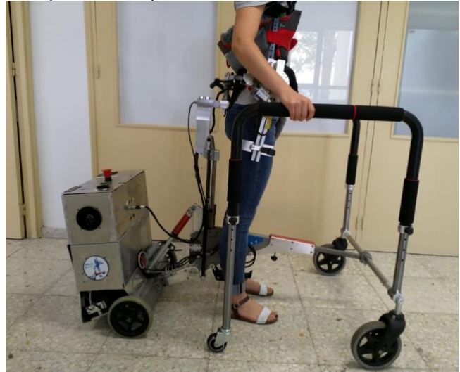
Figure 1. General view of the SWalker robotic platform
